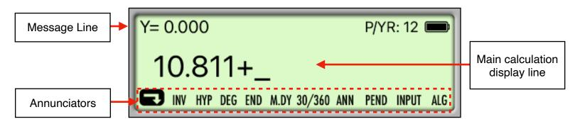
The RLM-10BX calculator's display has three areas: the message line, the main calculation line and the annunciators line.
