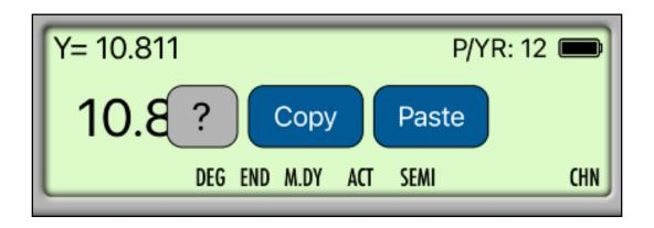
The "?" button turn on the quick help hint for for a short description of any keyboard or menu button action. As an example, in the following picture, the quick help for the "OPT" key is shown. To get back to the normal display, simply touch the display again.
